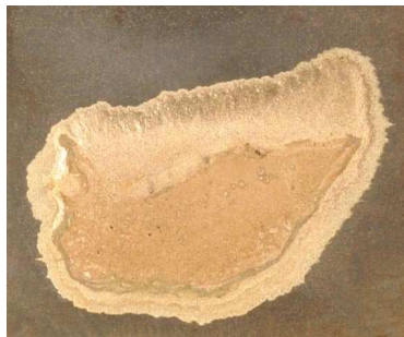
Fig 1(b): Here again the after testing sample shows evidence of interfacial corrosion attack. However the level is much lower than that experienced by Sample A . This is due to the presence of Nickel in Sample B , but note that attack has still occurred!
