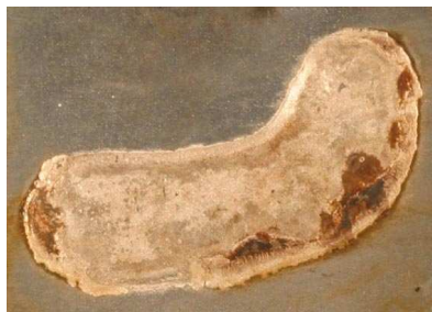
Fig 1(c): There is no evidence of interfacial corrosion in the ' after testing ' condition of Sample C , the very thin streak brown at the base of the alloy 'pool' and on its surface is mainly due to presence of manganese in the filler material: this is also visible in the ' before testing ' picture!
