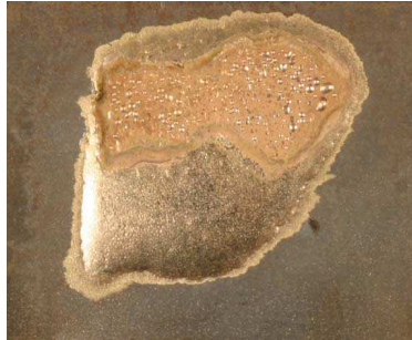
Fig 1(a): The thin line of a brown deposit at the edge of the brazing alloy that has formed in the after testing picture is a sure sign that the interface between the filler metal and the stainless steel is being attacked by 'interfacial corrosion'
