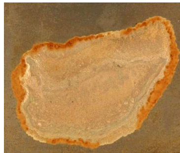
Fig 1(b): Here again the after testing sample shows evidence of interfacial corrosion attack. However the level is much lower than that experienced by Sample A . This is due to the presence of Nickel in Sample B , but note that attack has still occurred!
