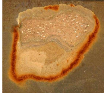
Fig 1(a): The thin line of a brown deposit at the edge of the brazing alloy that has formed in the after testing picture is a sure sign that the interface between the filler metal and the stainless steel is being attacked by 'interfacial corrosion'
