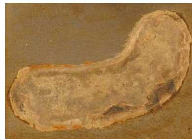
Fig 1(c): There is no evidence of interfacial corrosion in the ' after testing ' condition of Sample C , the very thin streak brown at the base of the alloy 'pool' and on its surface is mainly due to presence of manganese in the filler material: this is also visible in the ' before testing ' picture!
